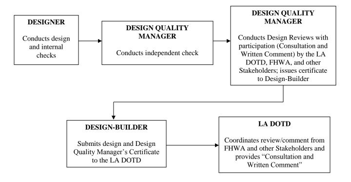
The Design-Builder and the LA DOTD will follow the process shown in Figure 111-11B for As-Built Plan Design Reviews.
